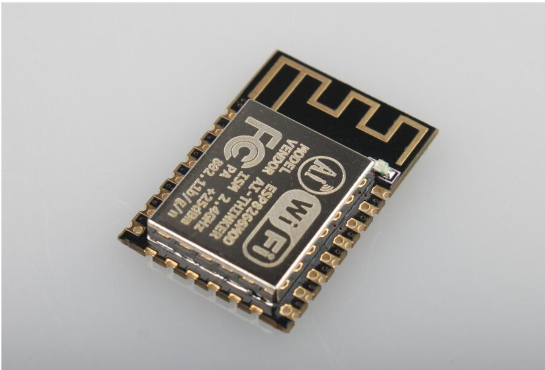
Figure 2 [Module Pin Counts, 18 pin, 16.0 mm x 24.0 mm x 3.0 mm]
