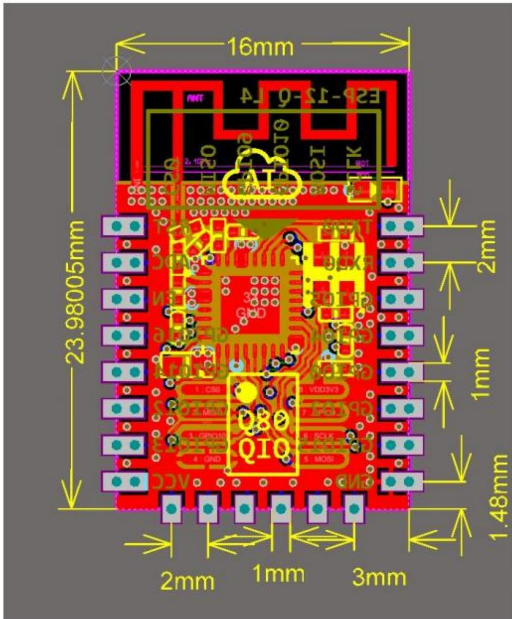
Figure 3 Top View of ESP-12F WiFi Module
